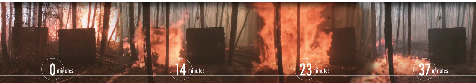
Simulated Forest Fires test the real world performance of FireMesh in protecting structures
