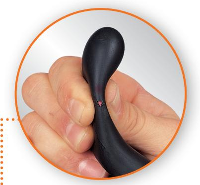
Damage shown here is due to wood and metal splinters and other sharp objects.
