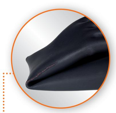
The strain on rubber at a folded point is equal to stretching the rubber to twice its length.
