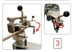
Undo the two knurled nut to release the conductor roller gate and drop down so the conductor or rope can be installed.
