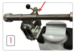
Place the roller on the insulator, with the twin horizontal & vertical rollers facing the angle of the conductor.
