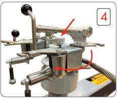
Complete the stringing and tensioning process, open the roller gates as in step 3.
