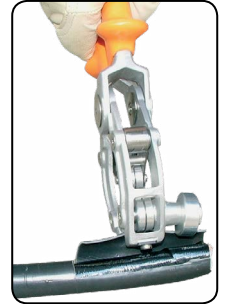
Stripping of Sheath
