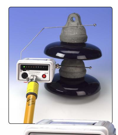
This product can be hand held for convenient testing of de-energised insulators in store yards, reclaim areas and in the field just prior to installation of insulators on the line. The tester is equipped with a universal spline for use with a hotstick allowing for convenient energised testing of insulators immediately prior to live line work. It is capable of testing insulators in a string at all voltage levels.
